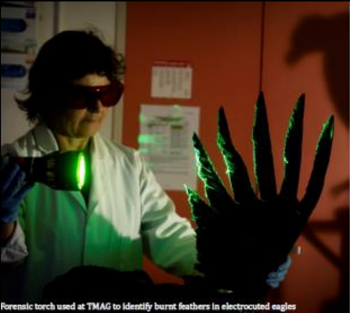
Forensic torch used at TMAG to identify burnt feathers in electrocuted eagles
